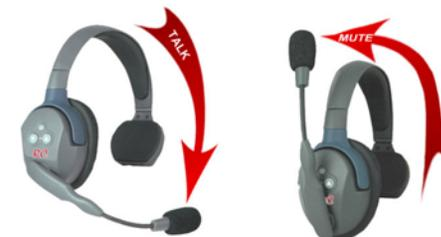
Microphone mutes automatically when boom is set to UP position.
